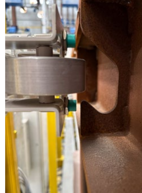
Reader for binary coding on the hardening grid
