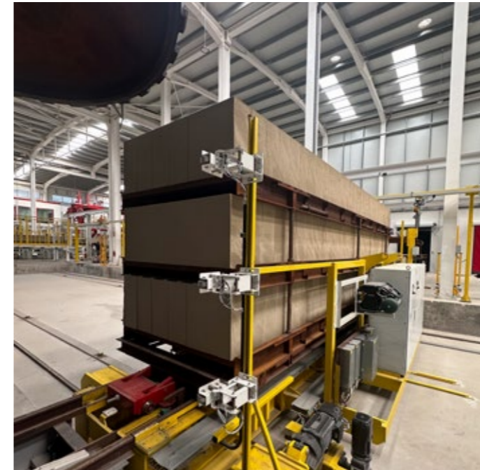
Cakes on tagged hardening grids on the way to hardening
