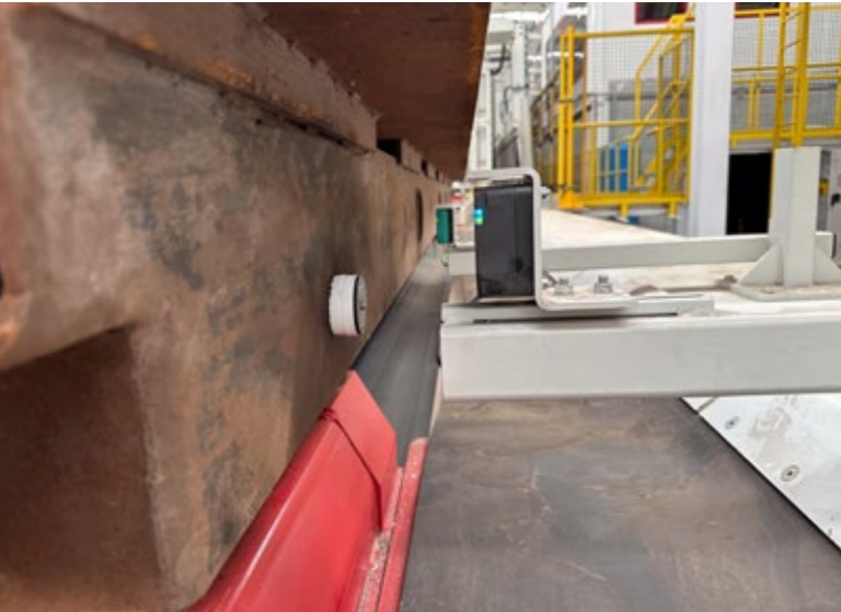
Mould side part tagged per RFID chip
