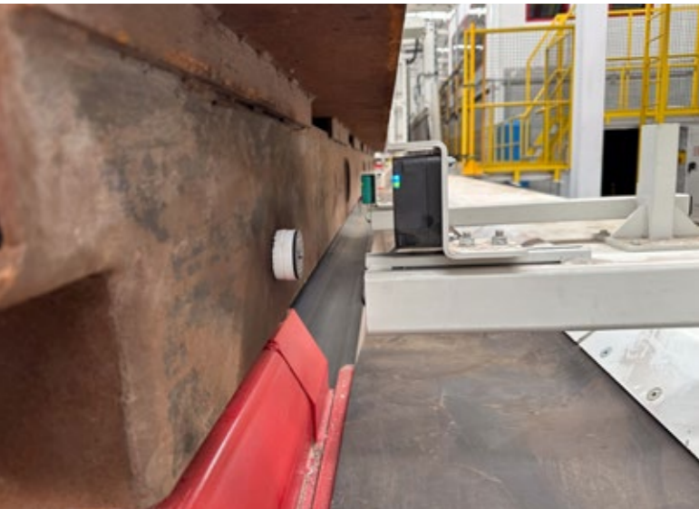
Mould side part tagged per RFID chip
